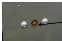
Press button on the back of machine, "ring", reset success. If there is no reaction, the thermostat is in reset position
