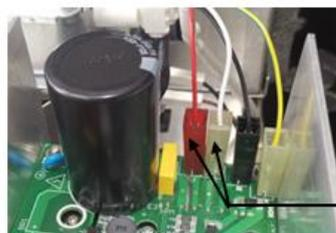
Unplug the terminals and measured the resistance between any two terminal :
