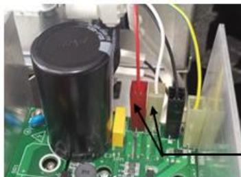
Unplug the terminals and measured the resistance between any two terminal :
