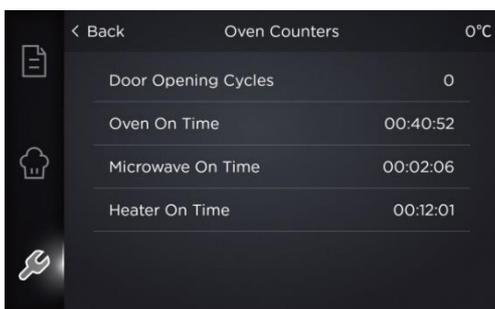
Check the "Oven Counters" to find the usage of components.
