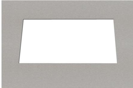
Making the cut in the surface in accordance with the installation drawing. **(Please only use detailed drawings)**. Use only suitable materials (stainless steel at least 3mm or granite).
