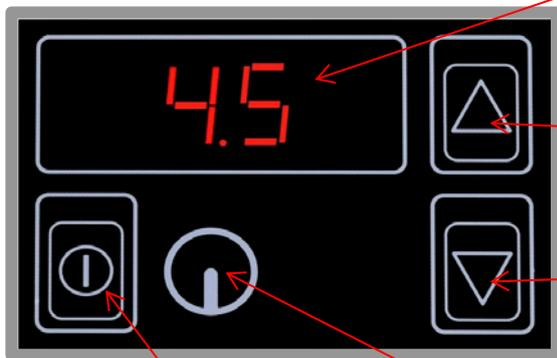
Digital display shows **Performance/temperature** (Precision +/- 1°C) or possible **Faults**
