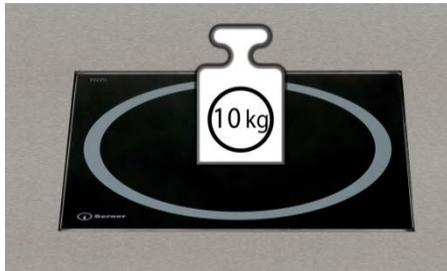
Place the glass ceramic plate in the center. (All around approx. 3 mm distance).
