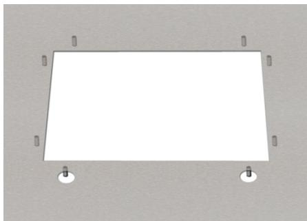
Install the bolts M6 on the bottom on the surface shown in the diagram (installation drawing) "mounting frame".
