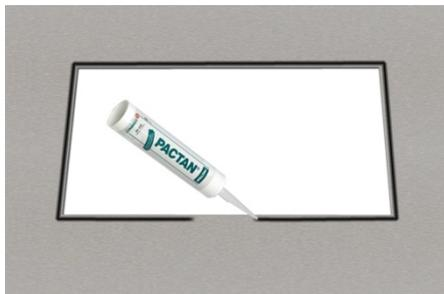
Assembling of the seal (pactan) without breaks to avoid a later leak in the seal.
