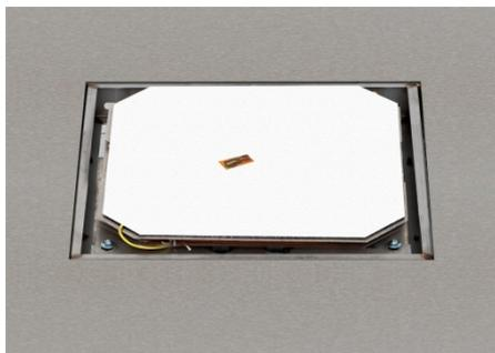
Insert the Induction unit from the top and install the cables. **Please follow this regulations: generator coil separate:** Feeler-, display- and control cables have to be installed separate from the coil and generator cables and if it`s possible be covered in a steel channel.
