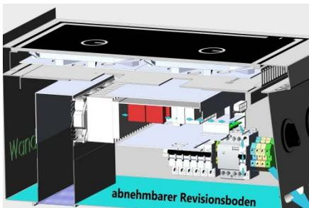
Install of the revisions plate (removable in case of service) with the cut out of the air channel (installation drawing) and connect with the adjustable air channel to the plate and seal of the edges with alu tape to protect it from greasy air.
