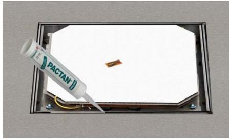
Applying a thin layer Pactan on the inner frame to fix the glass ceramic plate. Be careful in range of the display, to protect the display segment.
