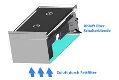
Assemble a switch face plate with air outlets Important: the air outlets should only open below to avoid liquid. To clean this unit don`t use splash water!
