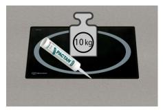
Fill the place between the glass ceramic plate and surface with excess pactan.
