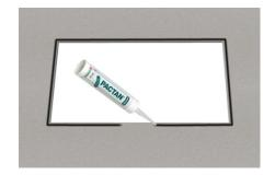
Assembling of the seal (pactan) without breaks to avoid a later leak in the seal.
