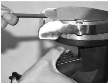
Sharpen the circular knife without teeth for approx. 1 to 2 seconds at a very flat angle from the bottom
