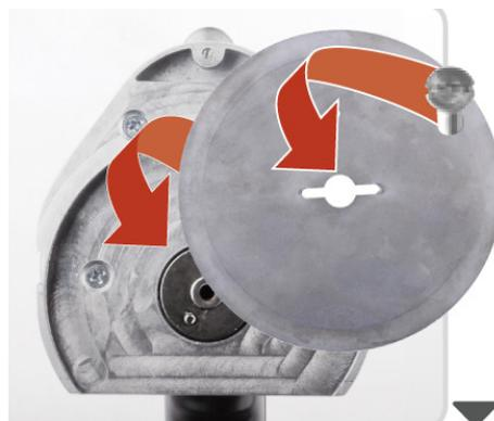
Insert the new knife, screw on
