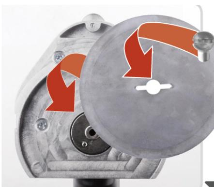
Insert the new knife, screw on the retention disk and fastening screw.
