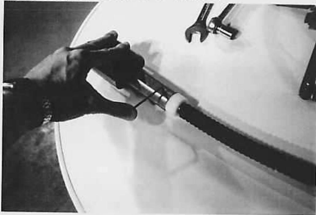
With a six sides key of 3, remove the 2 screws of the tool-holder, then pull out on the flexible.
